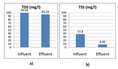
Figure 2. The mean values of influent and effluent wastewater TDS (a) and TSS (b) concentrations
