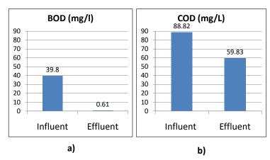
Figure 3. The mean values of influent and effluent wastewater BOD5 (a) and COD (b) concentrations
