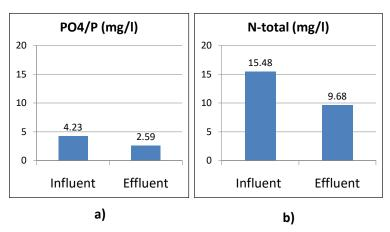
Figure 4. The mean values of influent and effluent wastewater PO4-P (a) and N-total (b) concentrations
