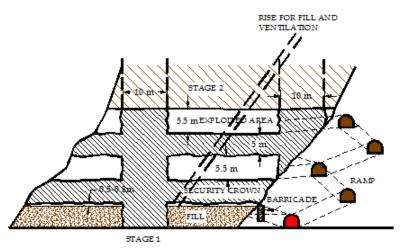
Figure 5. Preparing exploiting security crown and fill to exploited area
