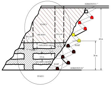
Figure 3. Presentation for two stage exploitation of ore body and forming security crown
