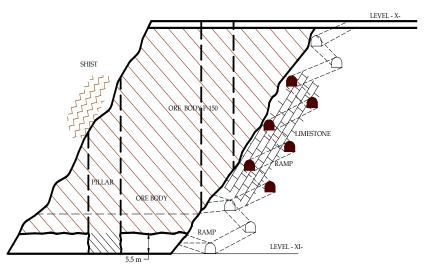
Figure1. Scheme of first phase of the exploitation of stope S-150
