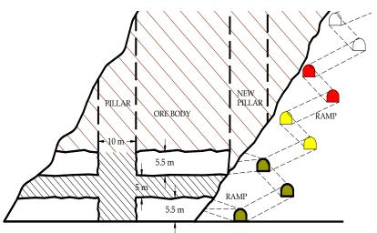
Figure2. System construction of safety pillars and crown during the exploitation phase
