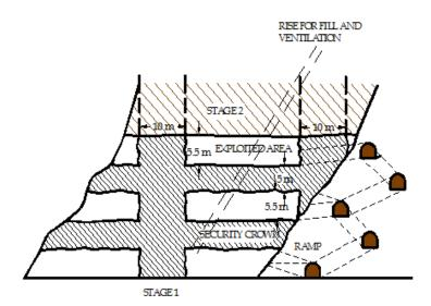
Figure4. Forming security crown and projecting to starting exploration.
