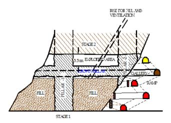
Figure8. Preparing exploiting secondary security crown and fill to exploited area
