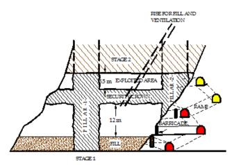
Figure7. First exploiting security crown and preparing for filling to phase two
