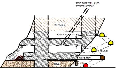
Figure6. Starting exploiting phase security crown
