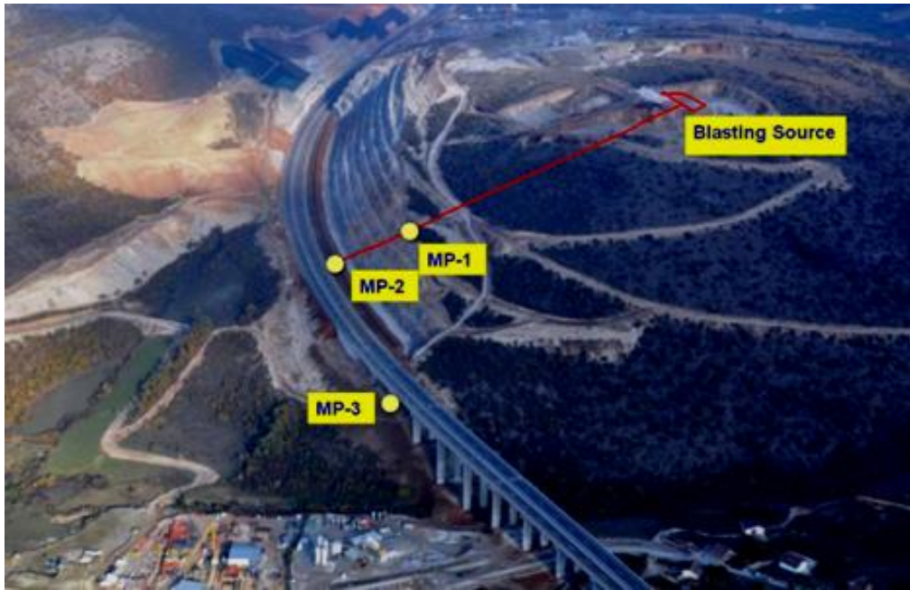
Figure 4. Measuring points and source of explosion
