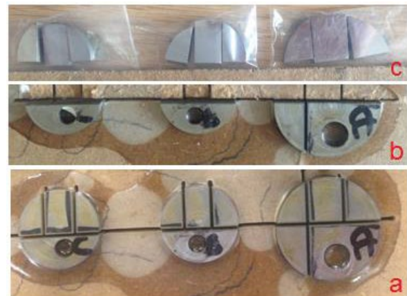
Figure 3. a) Dimensioning of the samples after the second cut. b) Unpolished parts, c) Polished parts
