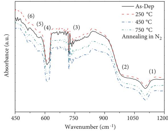
**Figure 1.** FTIR spectra of  $\text{Al}_2\text{O}_3/\text{Si}$  thin films at different annealing temperatures.
