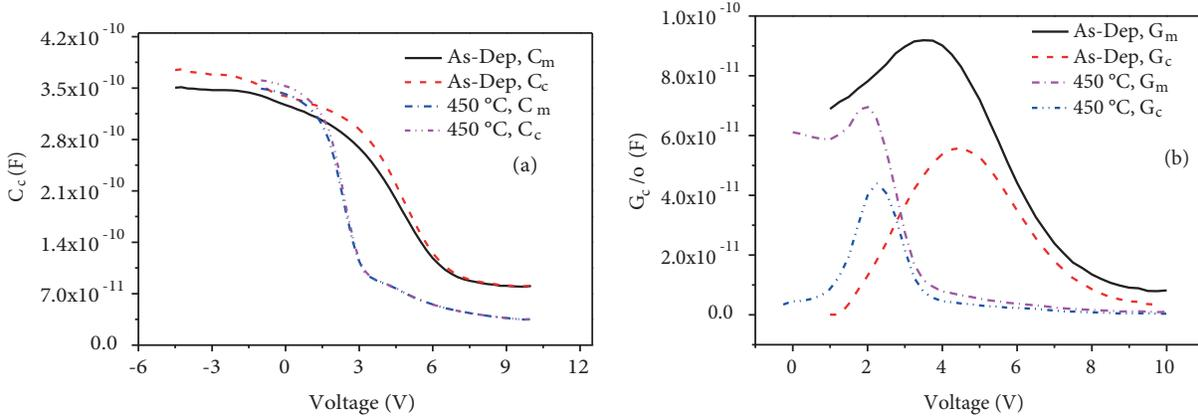
**Figure 5.** Variations of the corrected and measured a) capacitance and b) conductance for  $\text{Al}_2\text{O}_3$  MOS capacitors.
