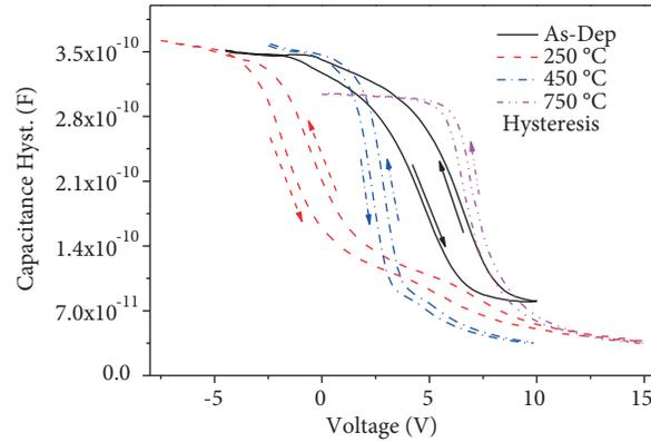
**Figure 4.** The capacitance hysteresis of Al<sub>2</sub>O<sub>3</sub> MOS capacitors depending on annealing temperatures.
