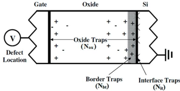
**Figure 3.** Important defect sites for the MOS structure that may influence electrical characteristics of the device [29].
