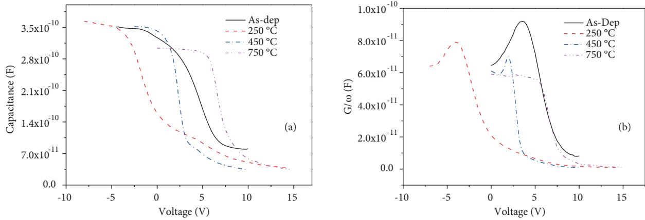
**Figure 2.** Variations of the a) capacitance and b) conductance curves of the  $Al_2O_3$  MOS devices after different annealing temperatures.
