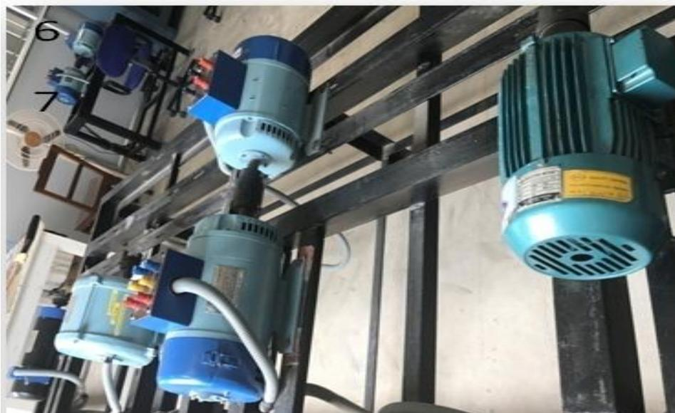
**Figure 8.** Overall machine arrangement along with alternator motor set
