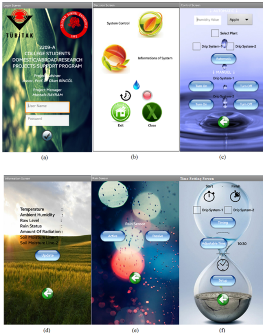
Figure 6. Sub screen of Android interface (a) Login screen, (b) Decision screen, (c) Control screen, (d) Information screen, (e) Rain sensor activation screen, (f) Clock setting screen
