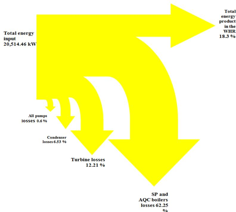
**Figure 5.** Energy flow diagram for the WHR system (reference state temperature and the atmospheric pressure are 15 °C and 101.32 kPa, respectively)
