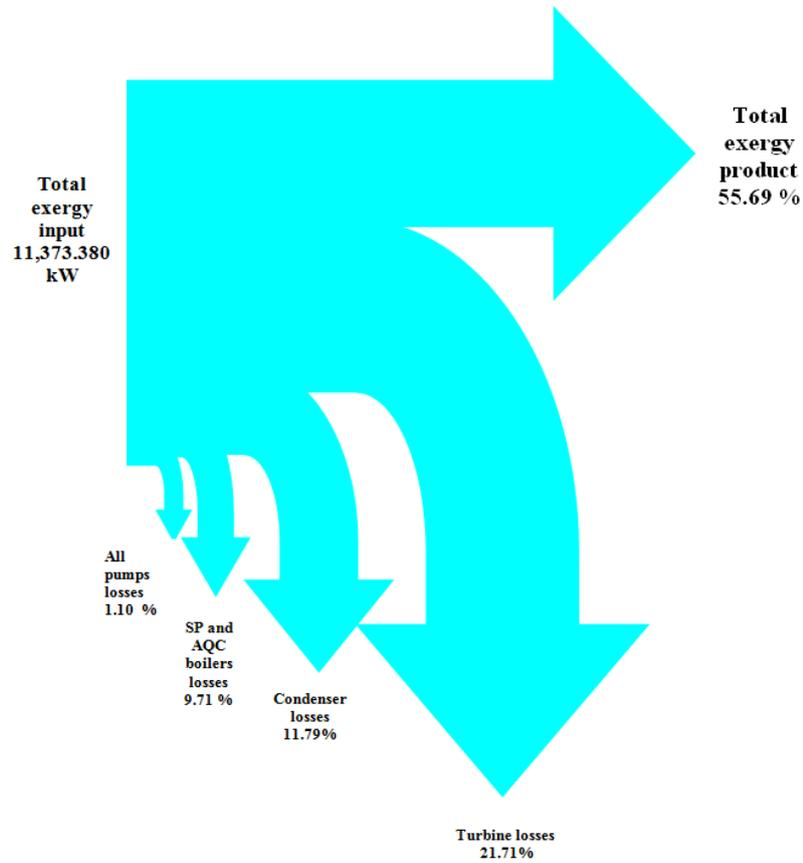
**Figure 6.** Exergy flow diagram for the WHR system (reference state temperature and the atmospheric pressure are 15 °C and 101.32 kPa, respectively)
