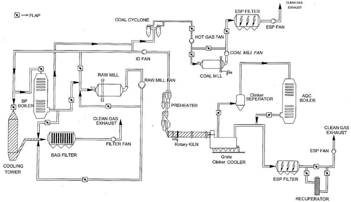
Figure 1. Energy Flow diagram in cement production system
