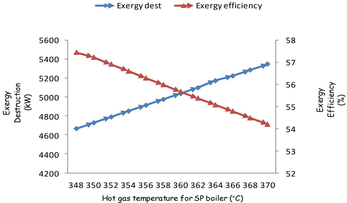
**Figure 8.** Variation of SP inlet gas temperature with exergy loss and efficiency of system
