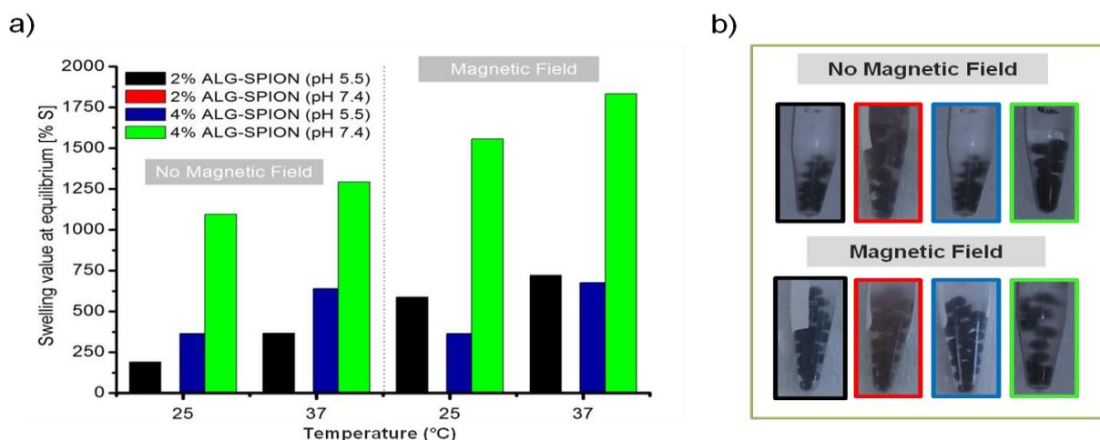
**Figure 4.** a) Effect of pH, temperature and magnetic field on the swelling value of the hydrogel at equilibrium depending on the initial alginate concentration of the ALG- SPION macrobeads and b) images depicting the effect of swelling after 24 hours at 37 °C (Frame colour of each image corresponds to legend color of the samples depicted in the graph. Experiments were carried out with 0.2 g/1 mL hydrogel
