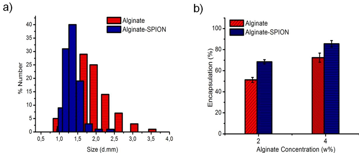
**Figure 3.** a) Size distribution and b) Cefazolin encapsulation efficiency of as prepared alginate macrobeads (2%) w/two superparamagnetic nanoparticles
