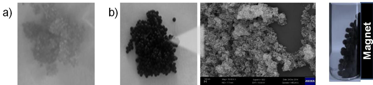
**Figure 2.** Photograph of Cefazolin encapsulating a) alginate macrobeads (2%) and superparamagnetic nanoparticle (SPION) embedded alginate macrobeads. FE-SEM image of SPION clustered on alginate bead surface and image demonstrating the magnetic properties of the resulting macrobeads
