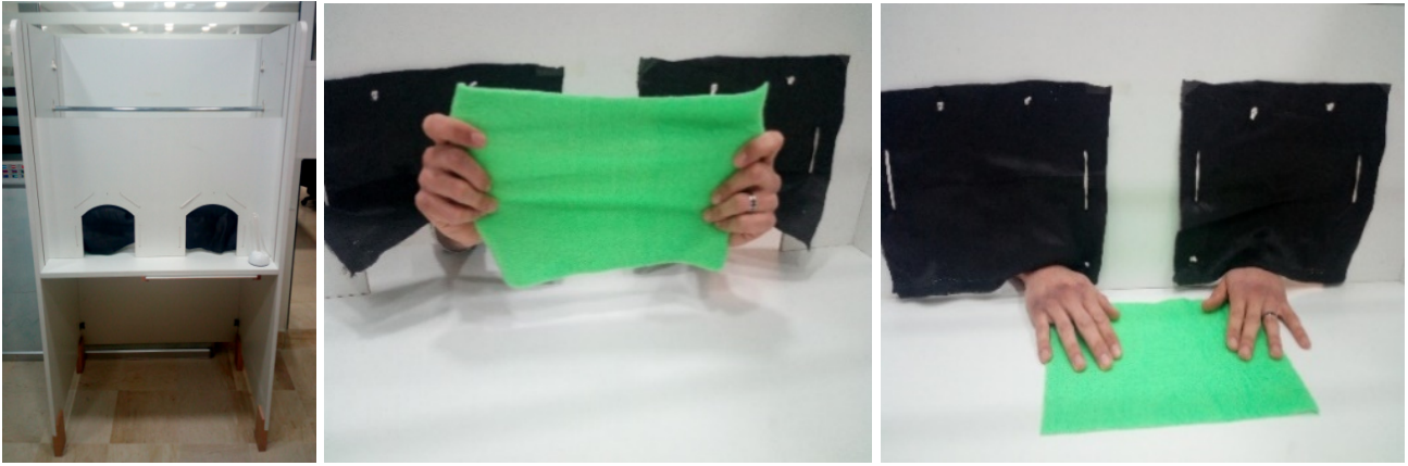
Figure 1: Developed assessment booth (sample and hand position from the back of the booth: animator side).
