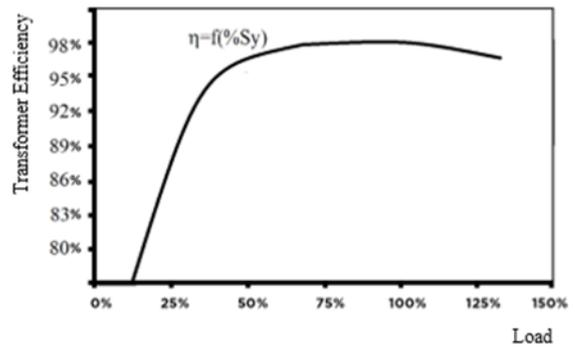
Figure 4. The change of 500-2000 KVA load transformer for  $\eta=f(\%S_y)$
