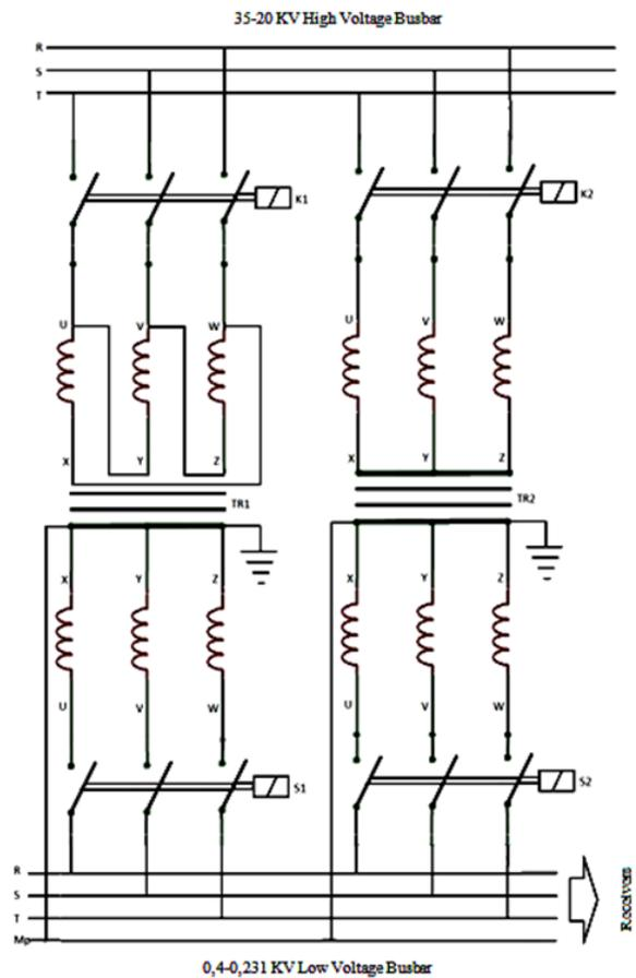
**Figure 2.** Parallel load transfer of transformers
