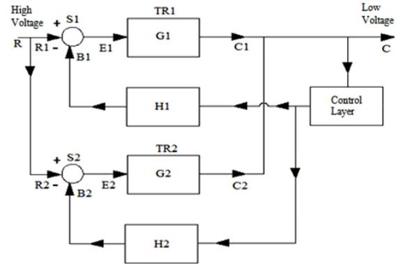
**Figure 1.** Energy efficiency based dual transformer control
