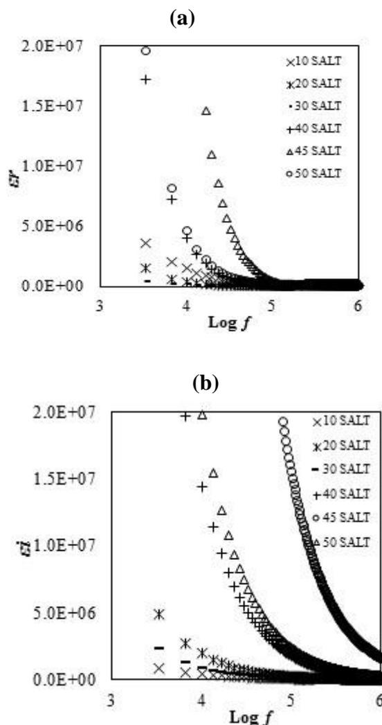
**Figure 3:** a) Real part of dielectric constant b) Imaginary part of dielectric constant, as a function of frequency for selected samples.
