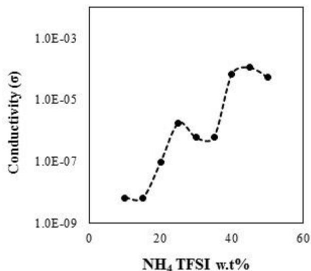
**Figure 2.** Variation of ionic conductivity as a function of NH<sub>4</sub>TF concentration
