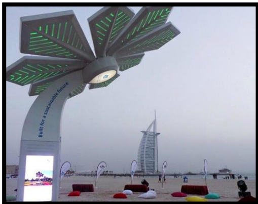
Figure 12: Solar powered palm tree (Robarts, 2015) in Dubai which provides wi-fi, by which phones and tablets can be charged, weather and sea conditions can be learned and which can be used as night lighting (Robarts, 2015).
