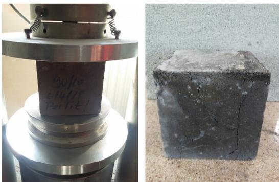
Figure 4. Compressive testing of foam concrete and
