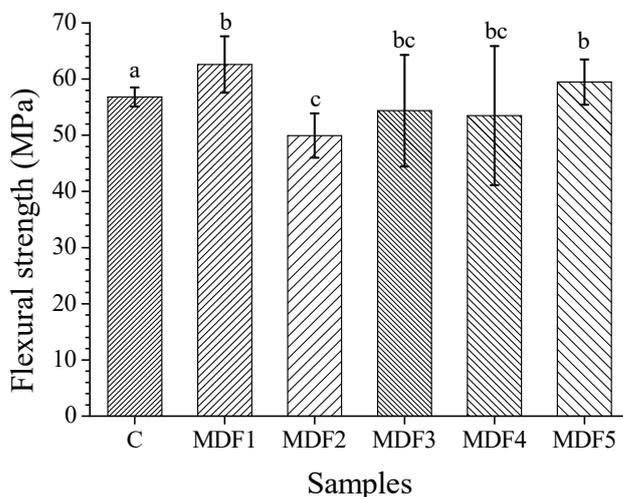
Figure 4. Flexural strength values of wood MDF powder-added PVC composites
