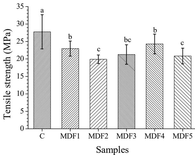
Figure 2. Tensile strength values of MDF powder-added PVC composites
