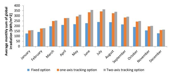
Figure 4. Monthly in-plane irradiation for Lefke at various mounting options
