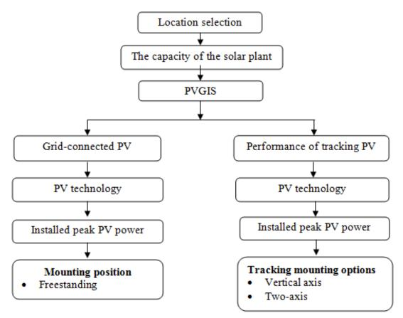
Figure 3. The framework of the simulation study using PVGIS
