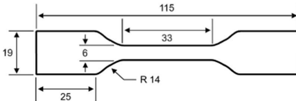
**Figure 5.** ASTM IV tensile test sample drawing.
