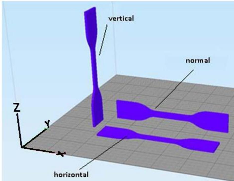
**Figure 3.** Printing positions of tensile test specimens.
