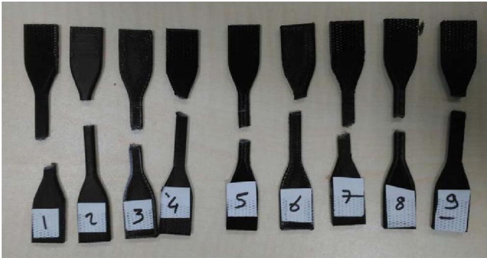
**Figure 6.** Appearance of test pieces after tensile test.
