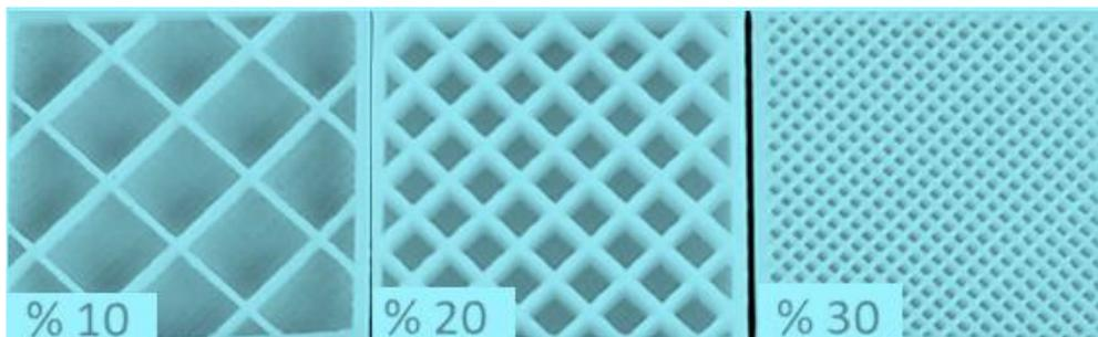
**Figure 4.** Display of internal filling ratio in parts.
