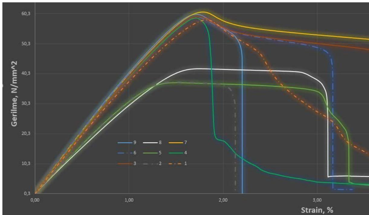
**Figure 7.** Tensile strain graph of tensile test specimens.
