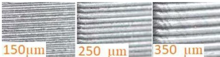
Figure 2. Display of layer height.
