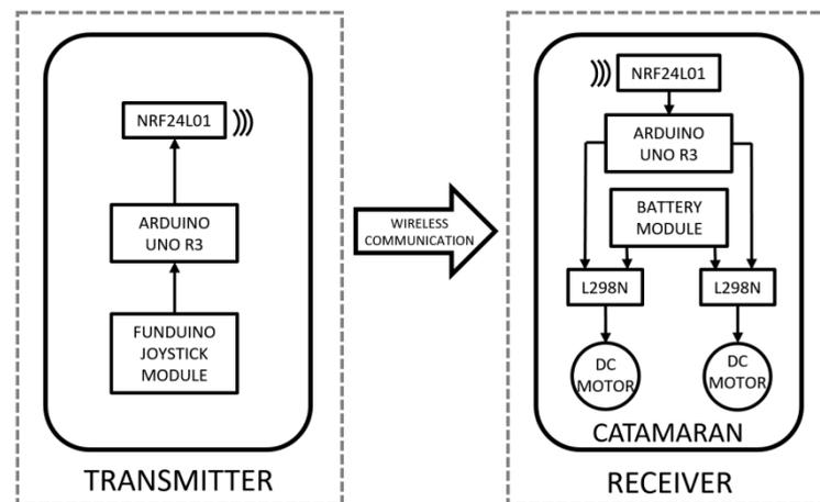
**Figure 6:** Catamaran remote control system diagram.
