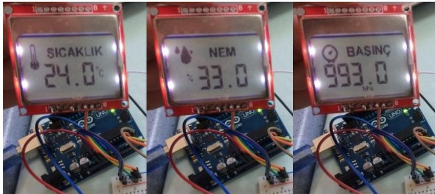
**Figure 8:** Weather station monitoring on LCD display.
