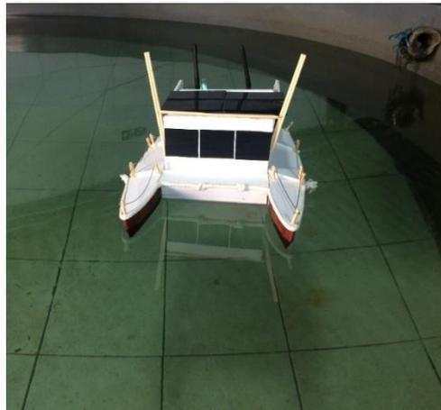
**Figure 12:** Water tests of model catamaran.
