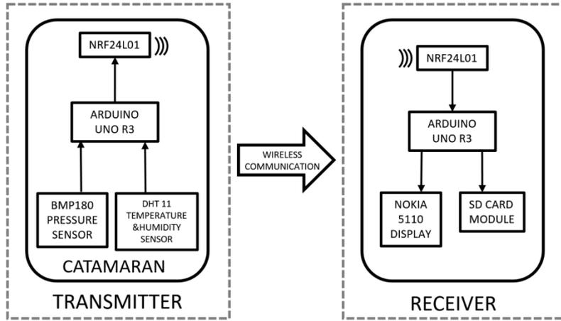
**Figure 7:** Catamaran remote control system diagram.
