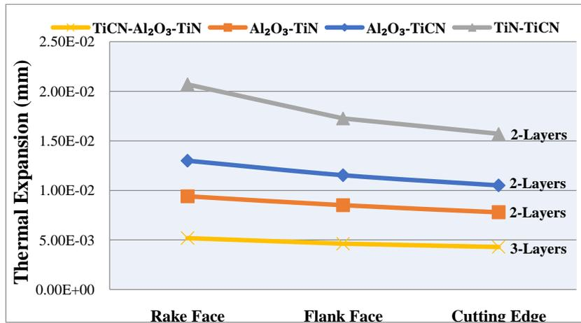
Figure 16: Dimensional thermal expansion comparison of multi-layer coatings
