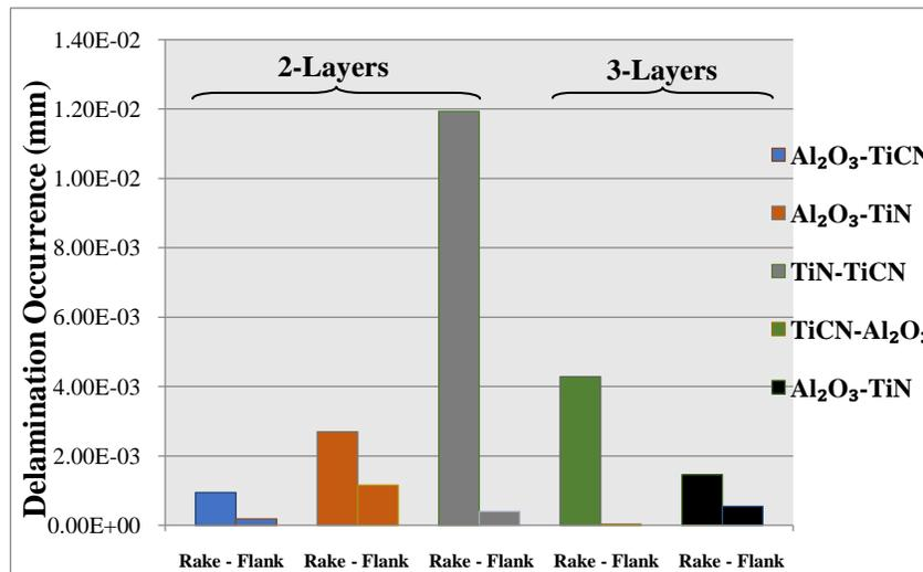
Figure 17: Delamination comparison in multi-layer coatings on the rake and flank faces (Z and X-Directions)
