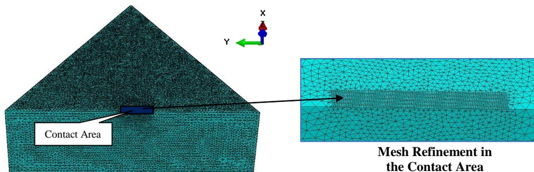
**Figure 4:** Created FE model and mesh refinement
