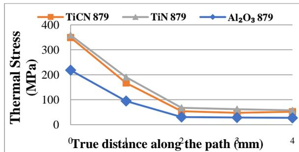
**Figure 8:** Thermal stress results for each coating material in HSM operation (Path-3)
