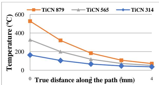
**Figure 6:** Temperature increment in single-layer TiCN coating (Path-2)
