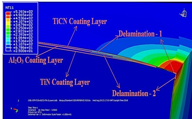
**Figure 15:** Appearance of delamination existence of TiCN-Al<sub>2</sub>O<sub>3</sub>-TiN multi-layer coating in HSM after cross-sectional view cut along the rake face
