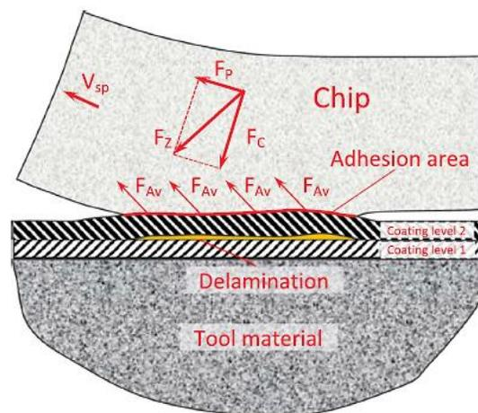
**Figure 3:** Delamination formation between multi-layer coating layers [28]
