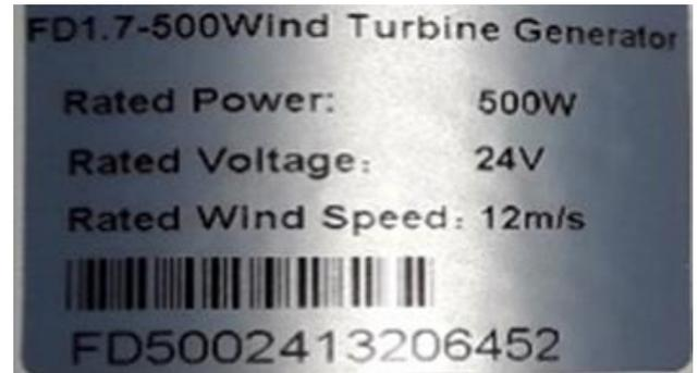
Figure 3. Wind turbine generator parameters
