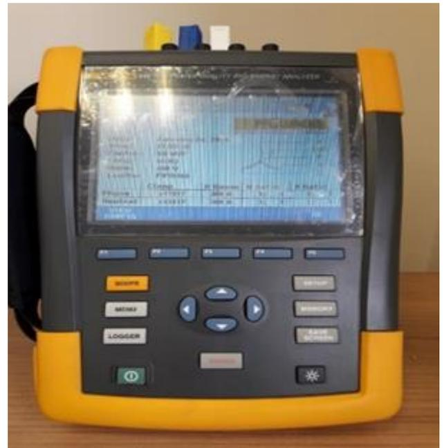
Figure 4. Fluke 435-II power quality and energy analyzer
