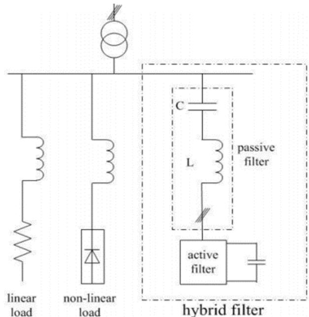
Figure 1. Hybrid harmonic filter [25]
