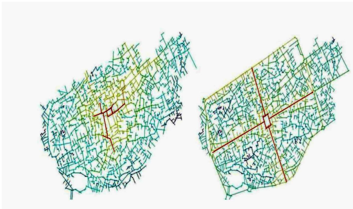
Figure 5. Integration of Kashan's routes before and after the construction of the automobile streets Obviously increased integration on the city after the streets were built and the connection was promoted slightly. Before and after the construction of the streets can be seen in Table 1,2,3 The major values for the five indexes of the core of the city. Mashhadizadeh Dehaghani, N. (1994), spatial Analysis of Space Syntax Symposium On Urban Planning in Iran. [17]
