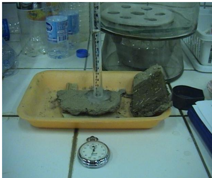
Figure 13. Time Dependent Water Absorption Test Absorption
