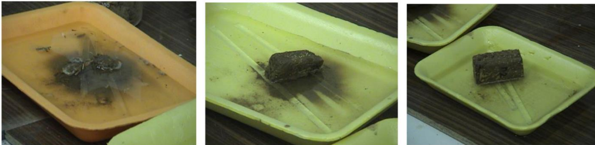
Figure 11. G1, K1, D1 Water Absorption of Samples by Capillarity
