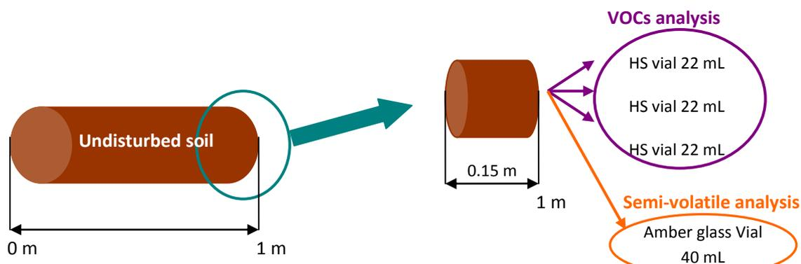
Figure 4. Sampling methodology and handling for hydrocarbons analysis
