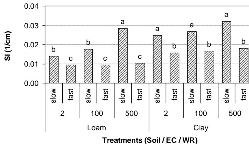
Figure 3. Structural index (SI) of the soils as affected by the treatments (EC-electrical conductivity, WR-wetting rate)
