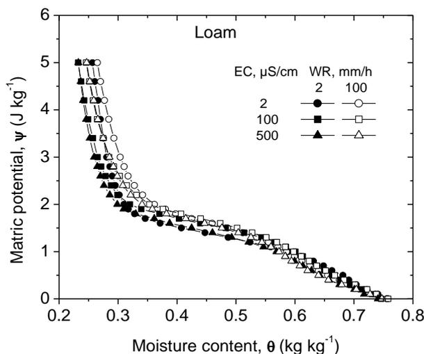
Figure 2. Water retention, of the loam soil aggregates wetted with different water quality.
