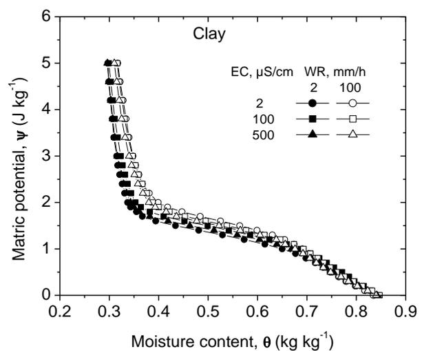
Figure 3. Water retention, of the clay soil aggregates wetted with different water quality.
