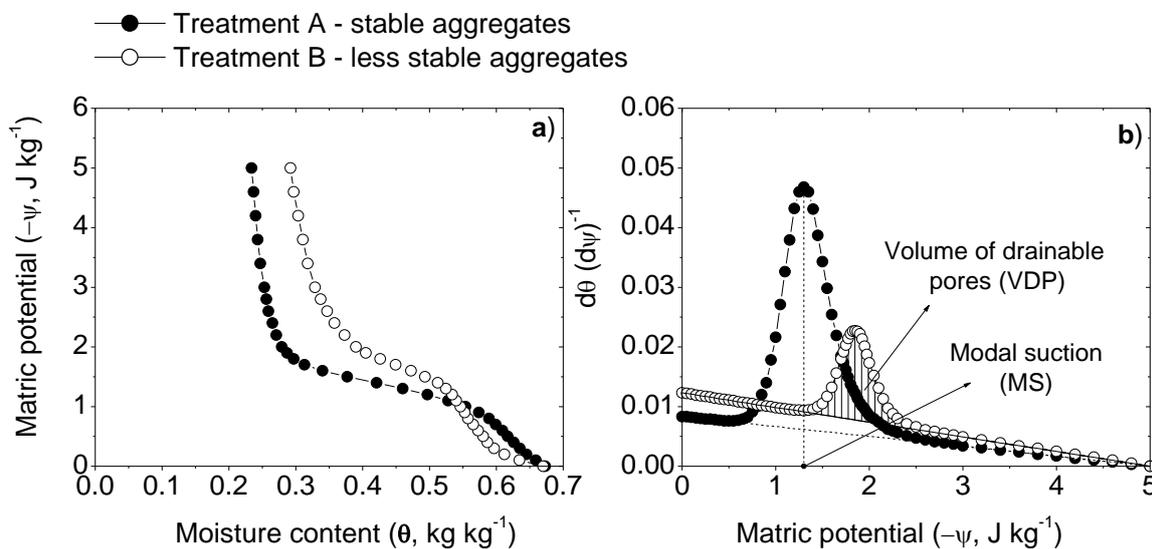
Figure 1.(a) water retention, and (b) specific water capacity curves of the clay soil aggregates subjected to fast wetting. The dashed baseline in the specific water capacity curve represents soil shrinkage line.
