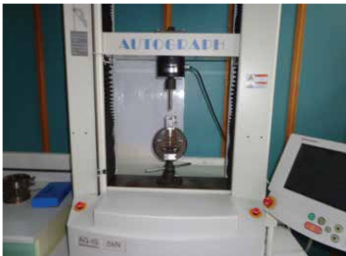
Figure 2. All specimens were stabilized and shear bond strength tests were performed in an universal testing machine.
