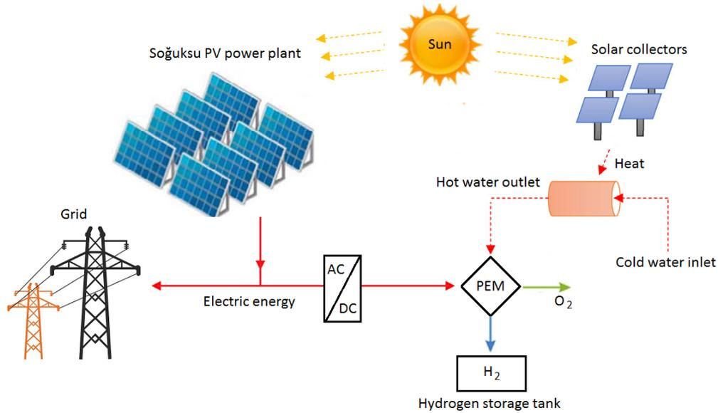
**Figure 1.** PV power plant aided hydrogen production system
