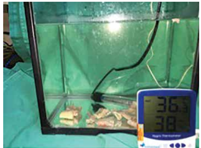
Figure 1. A thermal controller was used to adjust the temperature of the water close to the body temperature.
