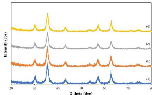
**Figure 2.** XRD pattern of (a) Fe<sub>3</sub>O<sub>4</sub> and (b) Fe<sub>3</sub>O<sub>4</sub>-OA nanoparticles, (c) Fe<sub>3</sub>O<sub>4</sub>-OA-CS and (d) Fe<sub>3</sub>O<sub>4</sub>-OA-GCS nanocomposites
