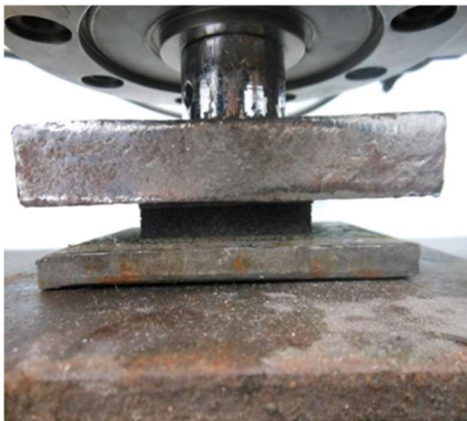
Figure 7. Flatwise compression test configuration
