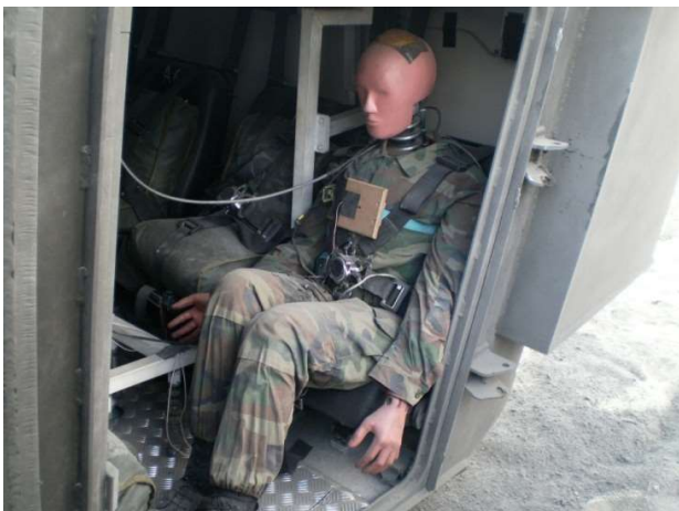
Figure 4 Hybrid-III dummy positioned for a mine blast test
