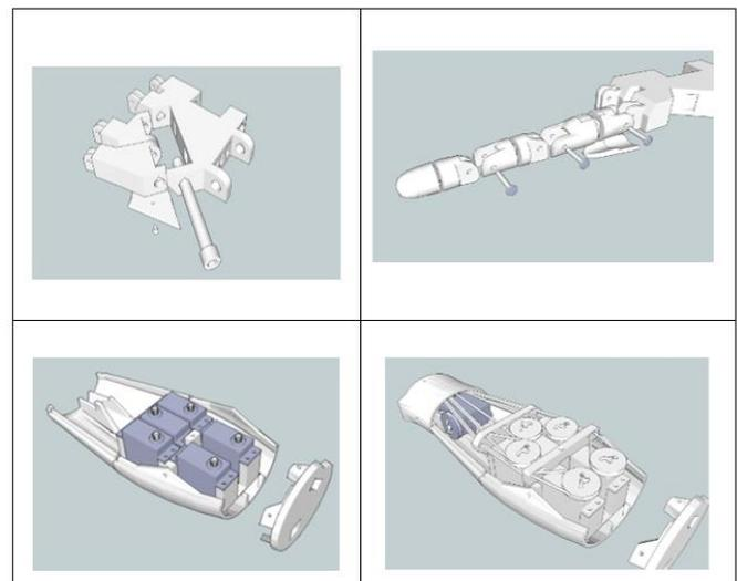
Fig.4. The stages of combining robot arm parts.
