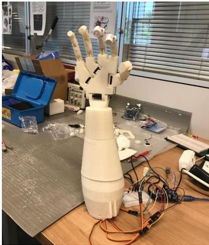
Fig.7. The implementation of the bionic hand..
