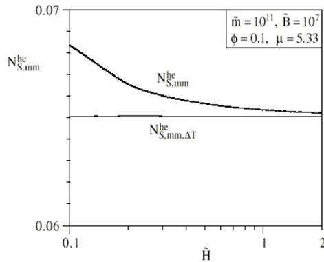
*Figure 5. The heat exchanger entropy generation rate minimized with respect to  $D_e/D_a$  and  $\tilde{L}_a$ , and its variation versus the third geometric parameter of the heat exchanger ( $\tilde{H}$ ).*
