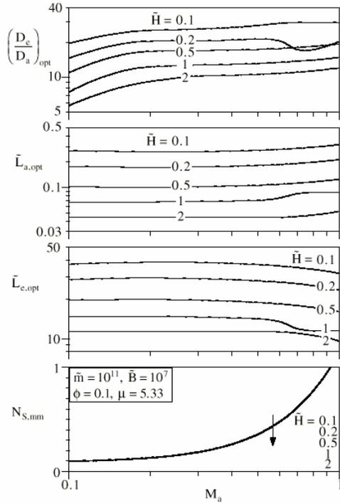
Figure 13. The effect of the approach Mach number on the optimized internal geometry of the heat exchanger.
