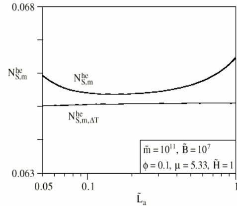
Figure 4. The variation of the minimized entropy generation rate with respect to the flow length  $\tilde{L}_a$ .
