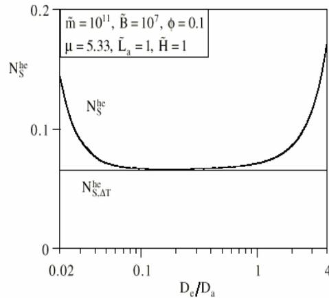
Figure 3. The first minimization of the heat exchanger entropy generation rate.
