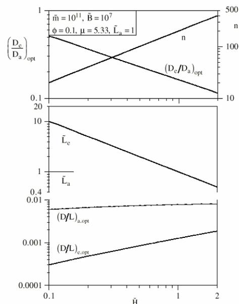
Figure 7. Optimal ratio of channel spacings and number of channels when  $\tilde{L}_a = 1$ , and the corresponding streamwise dimensions and channel aspect ratios.
