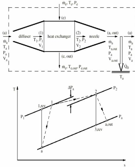
*Figure 1. Cross-flow heat exchanger with engine air on the hot side and ram air on the cold side, and the temperature-entropy diagram of the process undergone by the ram air stream.*
