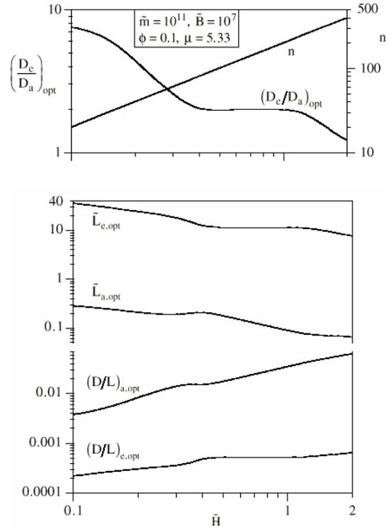
*Figure 12. The ratio of channel spacings, number of channels and slenderness ratios that correspond to the double minimization of the total rate of entropy generation.*
