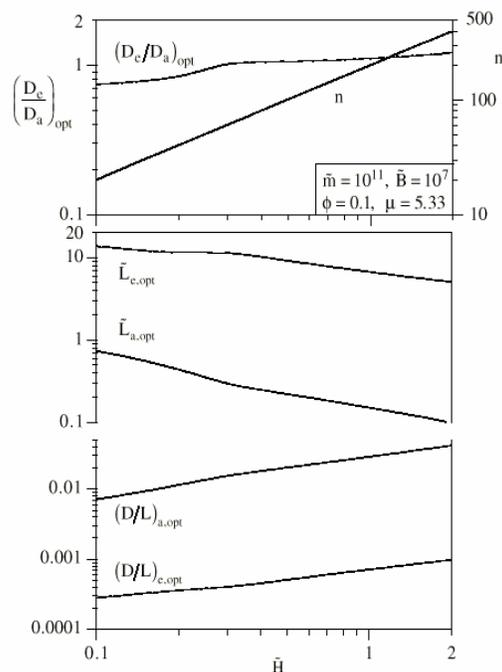
*Figure 6. The ratio of channel spacings, number of channels and channel aspect ratios that correspond to the system optimized in Fig. 5.*
