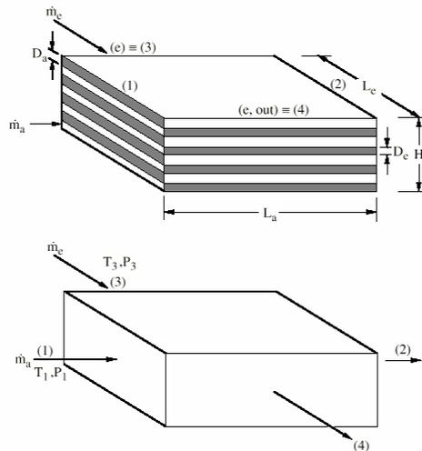
*Figure 2. Cross-flow arrangement consisting of parallel-plate channels.*
