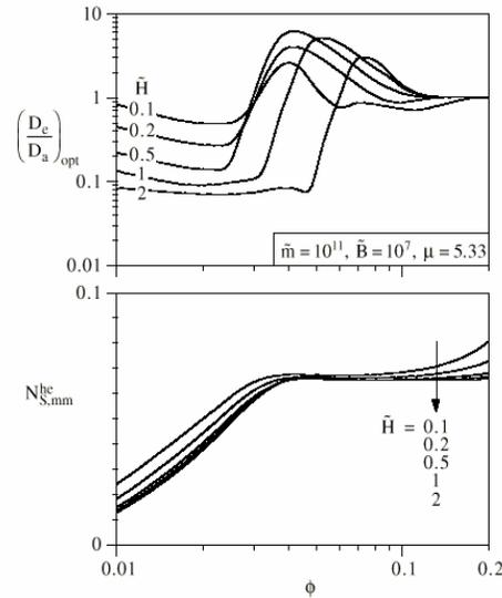
Figure 11. The effect of the volume fraction occupied by the solid parts of the heat exchanger core.
