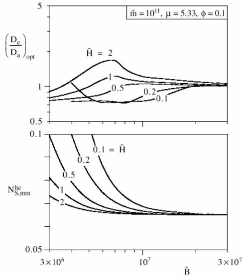
Figure 10. The effect of the heat exchanger core volume on the channel spacings ratio and the corresponding entropy generation rate.
