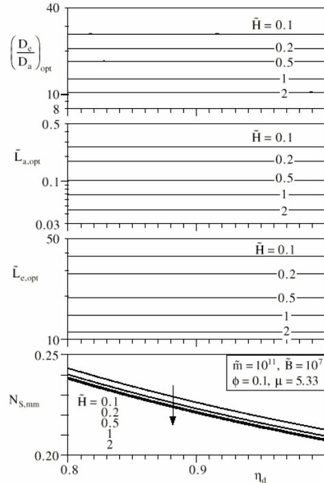
Figure 14. The effect of the diffuser efficiency on the optimized internal geometry of the heat exchanger.
