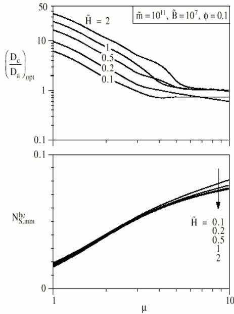
Figure 8. The effect of the capacity rate ratio on the ratio of channel spacings, and on the minimized entropy generation rate.
