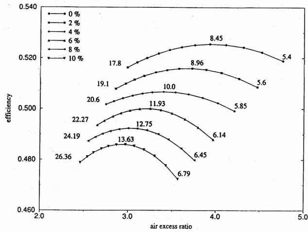
Figure 4. Efficiency of the power plant at the temperature of combustion gases 1200°C
