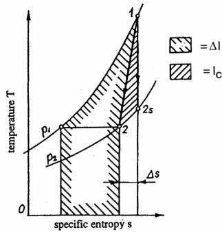
Figure 2. Influence of cooling of the blades on the work of turbine stage
