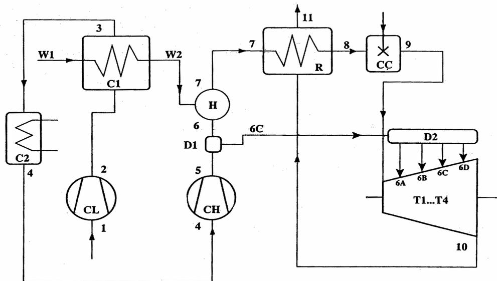
Figure 1. Scheme of the HAT power plant with cooling of turbine blades (CL, CH — low pressure and high pressure stage of the compressor, T1...T4 — stages of the turbine, C1 — interstage cooler and preheater of the injection water, C2 — external interstage cooler, CC — combustion chamber, H — humidifier of the compressed air, D — distributor of the cooling air, R — regenerative air preheater, 1...11 — streams of working fluid, W1, W2 — streams of injection water).
