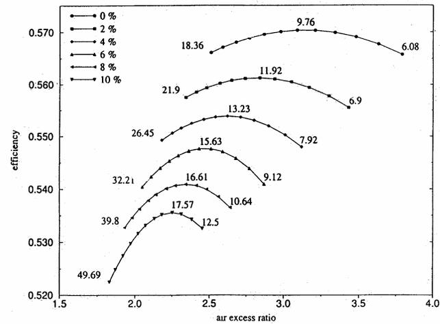
Figure 6. Efficiency of the power plant at the temperature of combustion gases 1400°C
