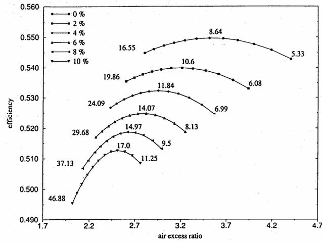
Figure 5. Efficiency of the power plant at the temperature of combustion gases 1300°C
