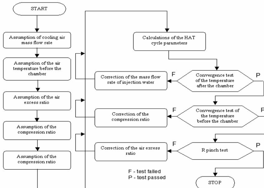
Figure 3. Block scheme of the calculations program
