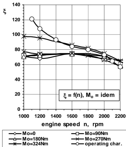
Figure 6. Resistance number  $\xi$  of the catalyt SZOP 07 – versus engine speed
