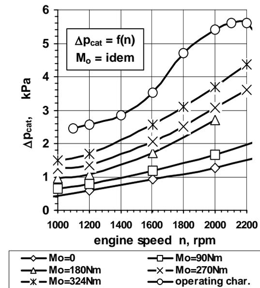
Figure 4. Pressure drop  $\Delta p_{cat}$  within the catalytic converter SZOP 07 – versus engine speed
