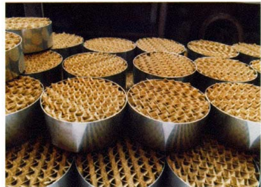
Figure 6. View of the ININ structured packing.
