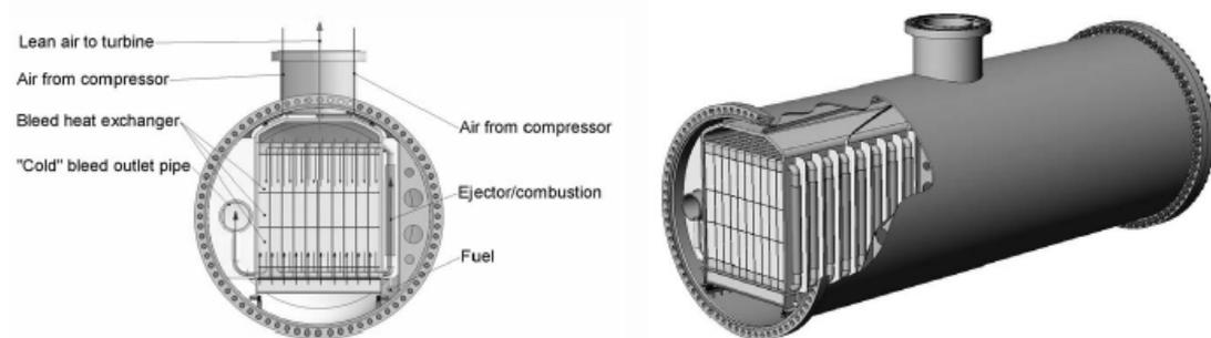
Figure 20. Design for an ITM reactor for the AZEP cycle (Sundkvist and Eklund, 2004).
