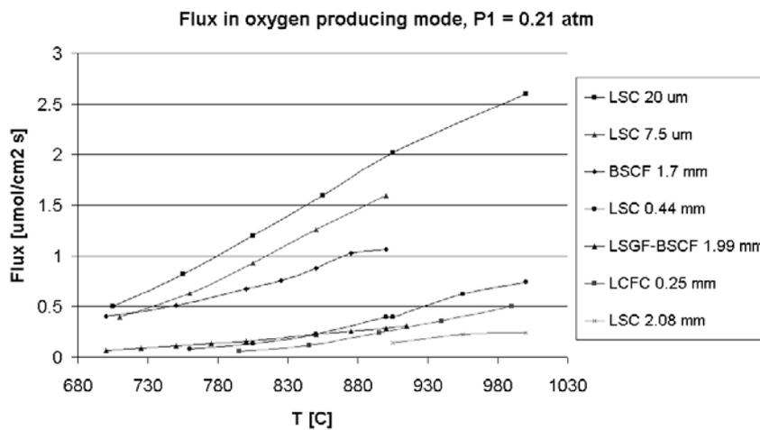
Figure 19. Actual non-normalised fluxes for membranes with different physical thicknesses. The names are listed in order of decreasing flux. (Foy and McGovern, 2005).
