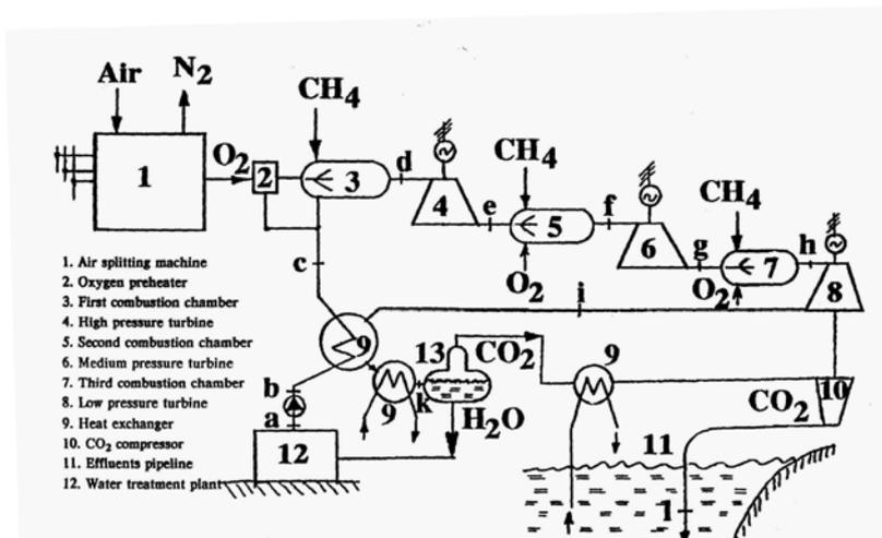
Figure 2. Power plant without exhaust gases (Yantovski, 1991).
