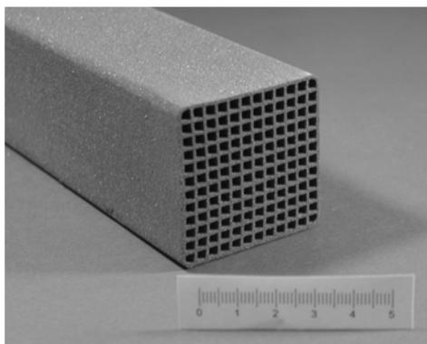
Figure 24. Membrane tested for oxycoal cycle (Renz, 2004).
