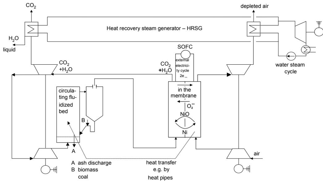
Figure 26. Coal or biomass fired zero emission cycle using an ion transport membrane as the oxygen carrier (Leithner, 2005).
