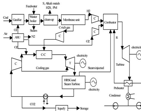
Figure 3. Flow diagram of IGCC system with steam-injected H<sub>2</sub>/O<sub>2</sub> cycle and CO<sub>2</sub> recovery
