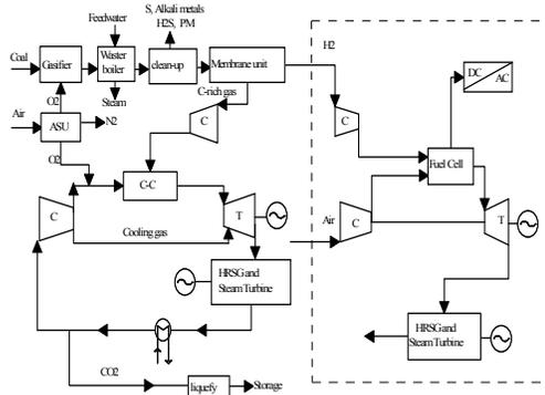
Figure 4. Flowchart of IGCC system with fuel cell combined cycle and CO<sub>2</sub> recovery
