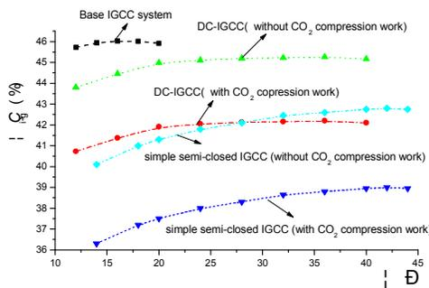
Figure 6.  $\eta_{ig}$  of different IGCC systems versus  $\pi$
