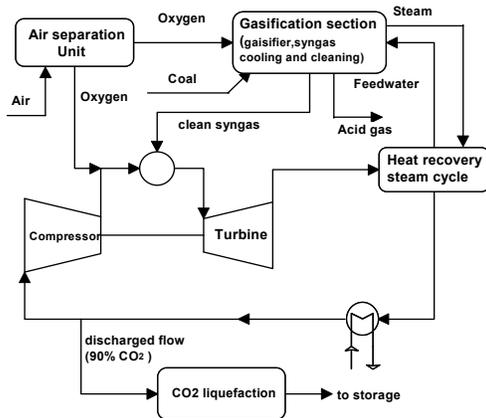
Figure 1. Flowchart of the semi-closed cycle IGCC system with CO<sub>2</sub> recovery
