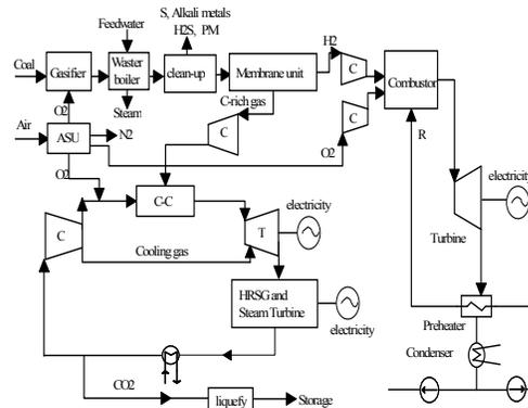
Figure 2. Flowchart of dual-cycle IGCC system with mixed H<sub>2</sub>/O<sub>2</sub> cycle and CO<sub>2</sub> recovery
