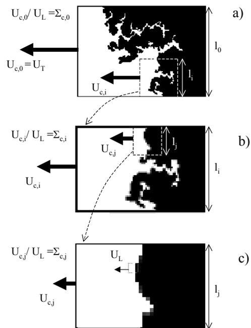
Figure 1: Scale-dependent behavior of turbulent velocity and roughness. a)  $U'/U_L = 2.12$ . Equivalence ratio  $\phi = 1.05$ , dilution percentage  $\delta = 15\%$ ; b). Part of front of Fig. 1a rescaled; c) Part of front of Fig. b rescaled. The fronts b) and c) are extracted from one “real” front obtained experimentally. They could correspond to real fronts obtained for smaller values of  $U'/U_L$  (scale covariance).
