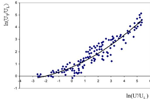
Fig. 4 : Experimental measurements  $\ln(U_T/U_L)$  vs  $\ln(U'/U_L)$  from Ronney et al. (1995). Second-order polynomial fit gives:  $\ln(U_T/U_L) = 0.048[\ln(U'/U_L)]^2 + 0.46\ln(U'/U_L) + 0.73$
