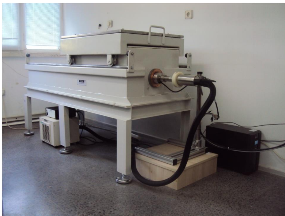
Figure 2. HPGe detector setup at NUBA used in present work
