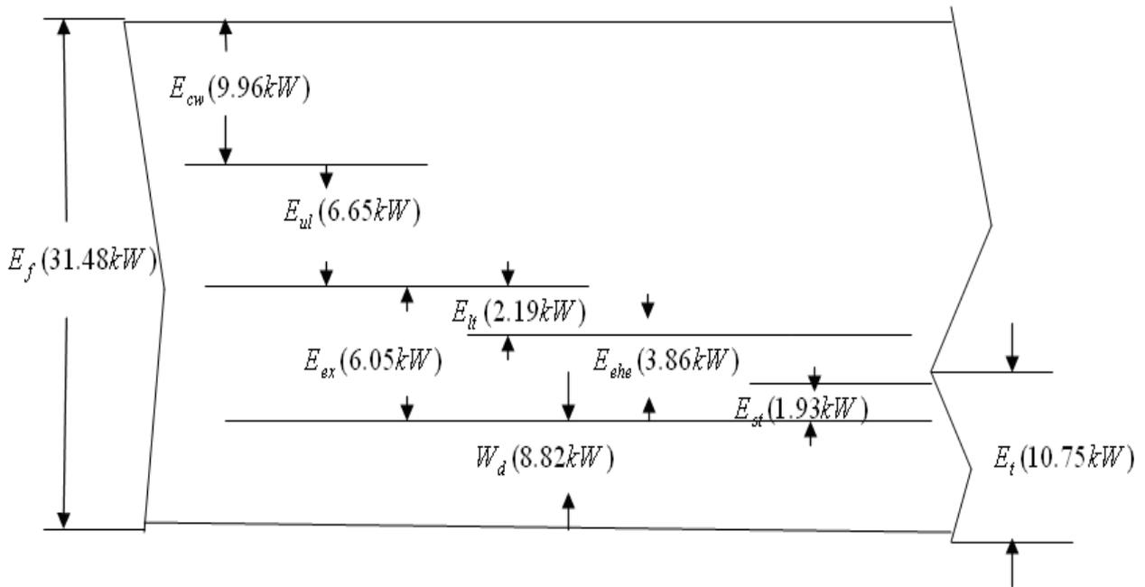
Figure 8. Energy Flow Diagram for the Diesel Engine Integrated with PCM system.
