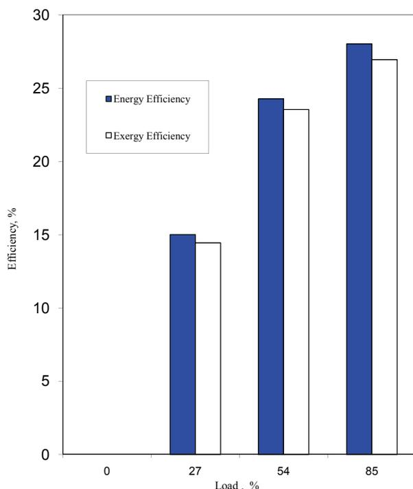
Figure 3. Efficiency of Diesel Engine with Load.
