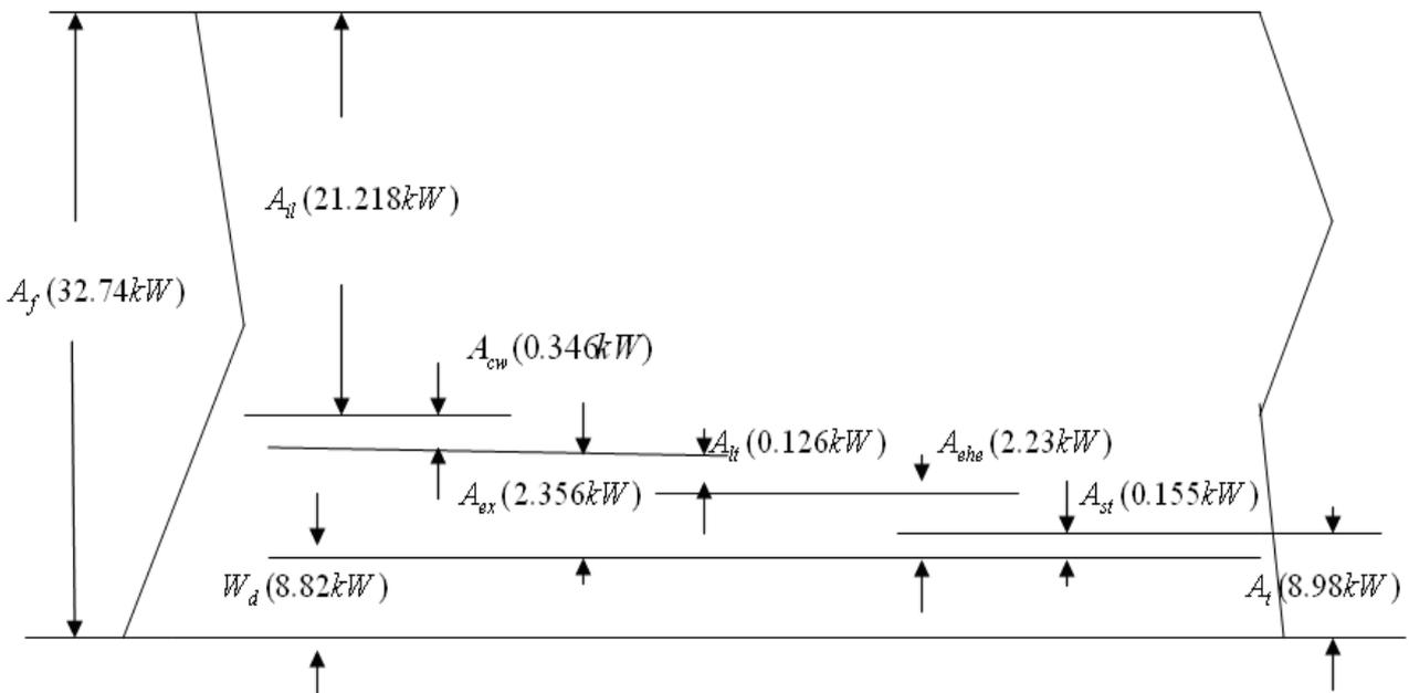
Figure 9. Exergy Flow Diagram for the Diesel Engine Integrated with PCM system
