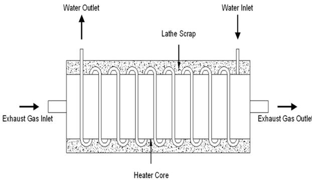
Figure 2. Schematic Diagram of Exhaust Heat Exchanger.
