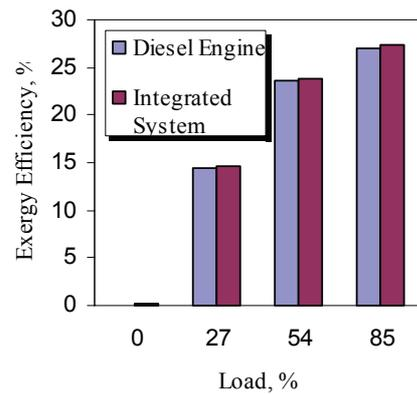
Figure 7. Exergy Efficiency of Diesel Engine and Integrated System.
