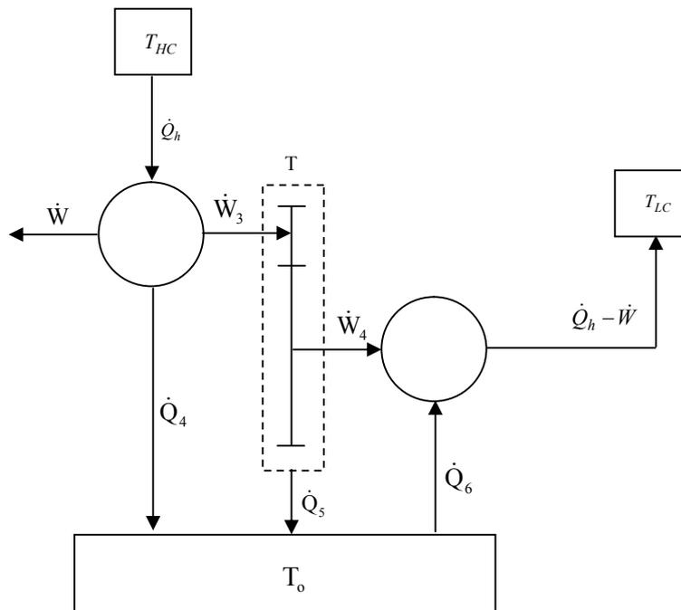
Figure 5. Equivalent model representing internal irreversibilities in the engine
