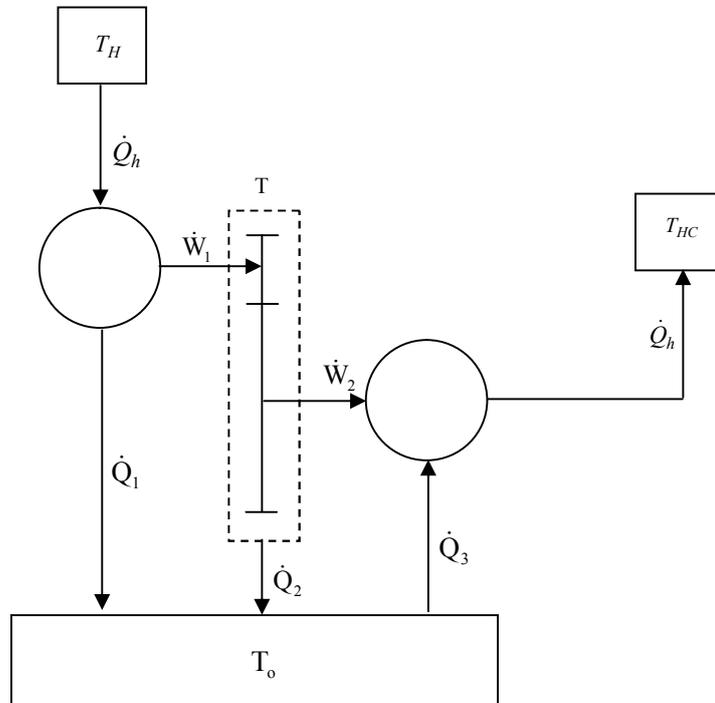
Figure 4. Equivalent model representing external irreversibilities caused by the hot heat sink
