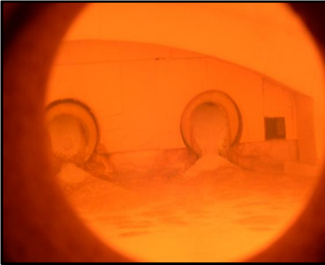
Figure 12. View into the GlasFLOX glass melting furnace (figure is in color in the on-line version of the paper).
