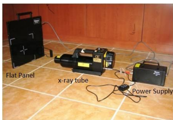
Figure 3. View of X-ray radiography system
