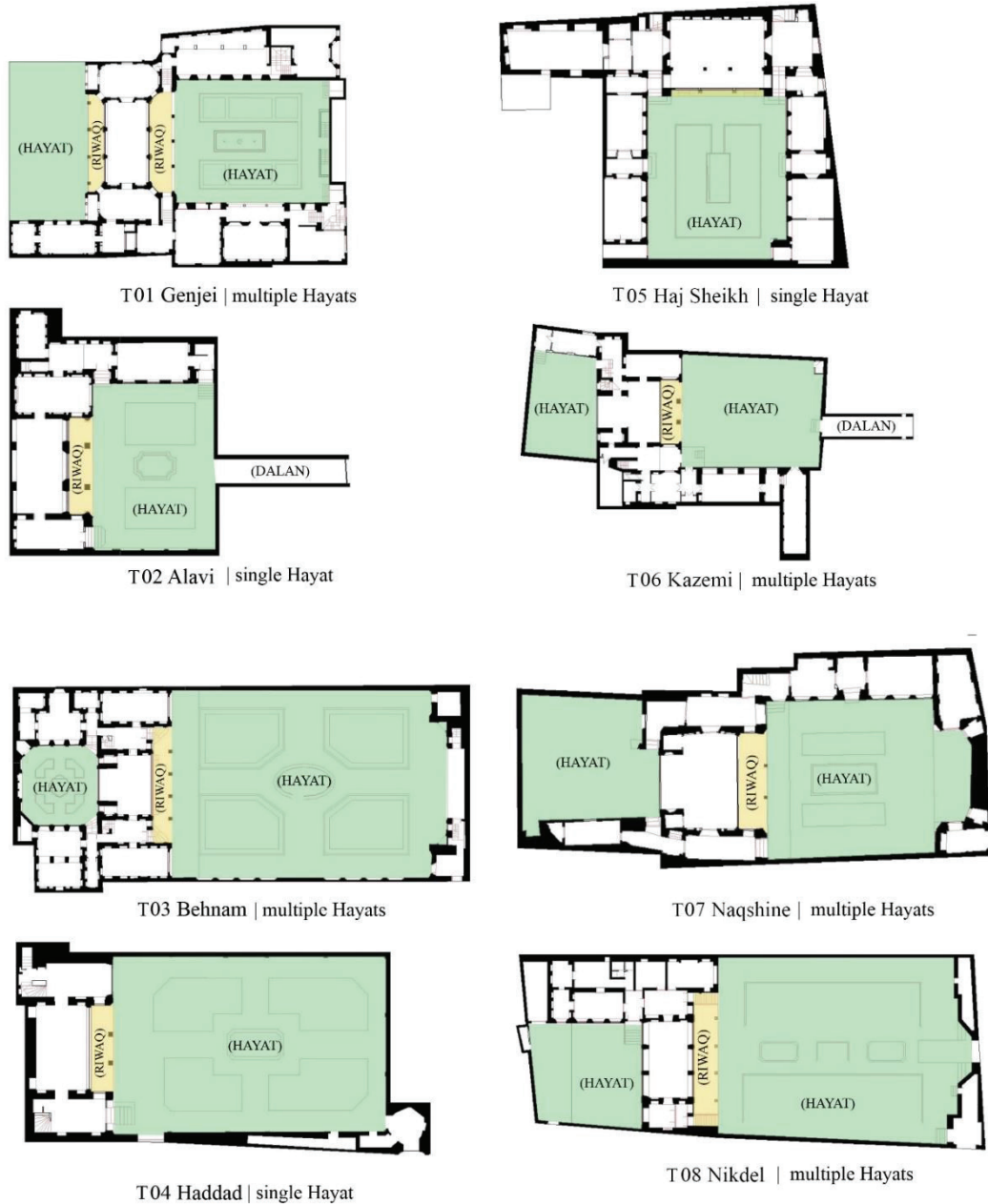
Figure 13. Plan charts of the selected samples for analysis of traditional Tabriz houses
