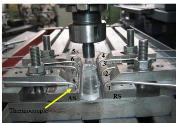
Figure 2. Friction stir welding device and test fixture with thermocouples
