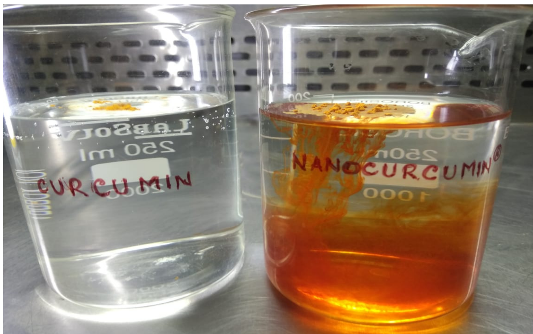
Figure 5. Solubility in water: left side- Only Curcumin, where the sample was not at all dissolving in water, it was floating on water surface; whereas in right side- Nanocurcumin is automatically dissolving in water.
