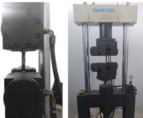
Figure 8. Tensile testing machine and test specimen
