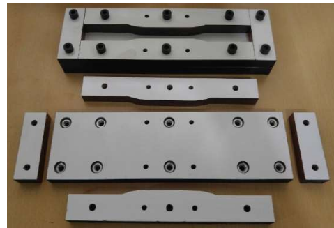
Figure 3. Molds for the tensile test specimens
