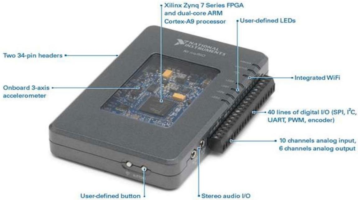
**Fig 1:** Image of Accelerometer Embedded in MyRio Device is acted upon by  $g$  force [13]. The resultant changes in the movement of the plate in relation to each other determined acceleration. Summarily, an accelerometer can be described as a transducer that converts mechanical stress or other forms of energy into an electrical signal [14]. A typical 3-dimensional accelerometer axis is shown in Figure 2 with each axis monitoring a specific activity of the vehicle.
