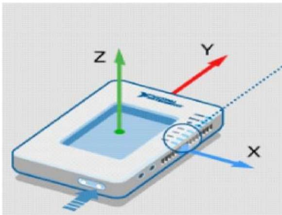
**Fig 2:** A Typical Accelerometer 3 D- Axis
