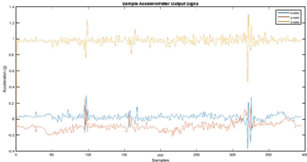
Fig 3: Sample Measured Road Surface Conditions Signals for each of the Accelerometer 3-D Axis
