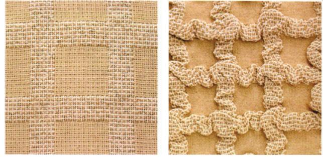
**Figure 5.** The fabric that has double weaving structure method with wool and rayon yarn woven and fulling by Pauline Verbeek-Cowart (12).
