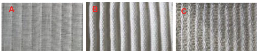
Figure 14. A) Appearance on the loom, B) Appearance after the relaxation of fabric (FRONT), C) Appearance after the relaxation of fabric (BACK)
