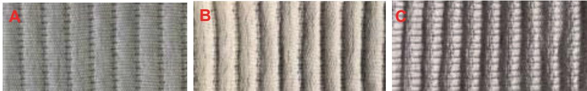
**Figure 19.** A) Appearance before caustic soda application, B) Appearance after caustic soda application (FRONT), C) Appearance after caustic soda application (BACK)
