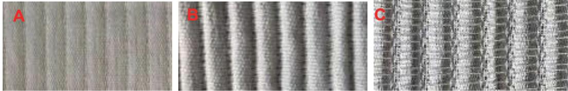
**Figure 18.** A) Appearance before caustic soda application, B) Appearance after caustic soda application (FRONT), C) Appearance after caustic soda application (BACK)
