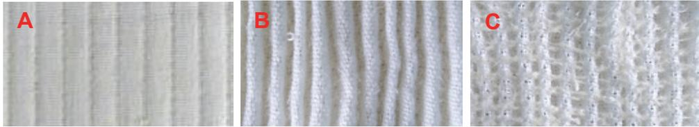
**Figure 16.** A) Appearance on before the fulling process, B) Appearance on after the fulling process (FRONT), C) Appearance on after the fulling process (BACK)
