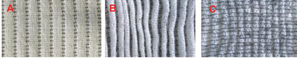
**Figure 17.** A) Appearance on before the fulling process, B) Appearance on after the fulling process (FRONT), C) Appearance on after the fulling process (BACK)
