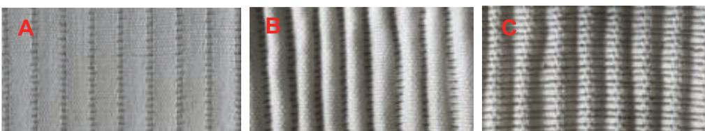
Figure 15. A) Appearance on the loom, B) Appearance after the relaxation of fabric (FRONT), C) Appearance after the relaxation of fabric (BACK)
