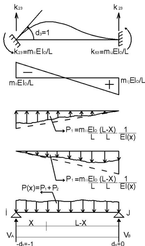
**Figure 3.**  $d_3 = 1$  loading and Mohr method
