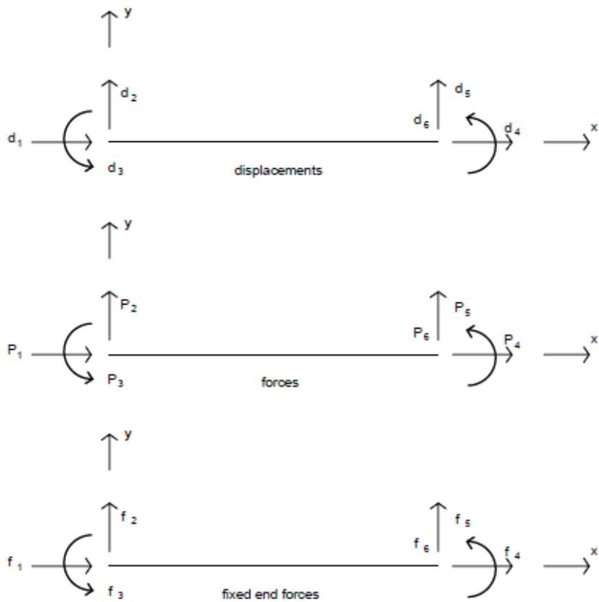
**Figure 2.** End displacements, end forces, and fixed end forces
