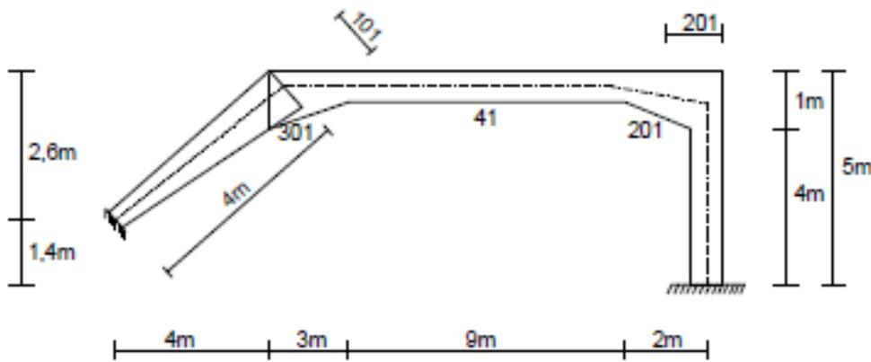
Figure 6. Example of variable cross-sectioned frame
